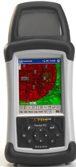
The TDS Recon handheld runs Windows Mobile 2003 software for Pocket PCs; meets MIL-STD-810F military standards for drops, vibration and temperature extremes; and is meaning it's impervious to water and dust.
